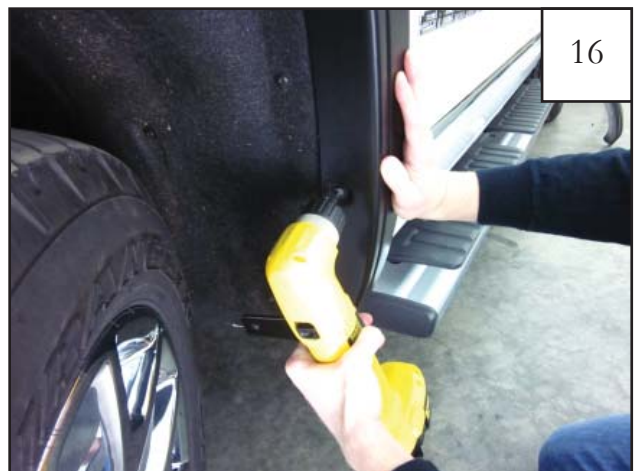
Install self-tapping screw (SW1-0066) into pilot hole drilled in step 13. Press flare towards vehicle while fully tightening. Note: This step not needed for models with factory installed mudflaps.
