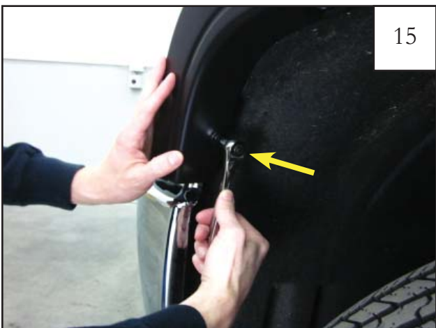
While holding Flare on vehicle, install factory screw removed in Step 4 through flare and into factory hole. Do not fully tighten at this time.
