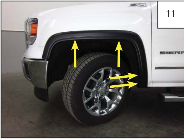
While holding Flare on vehicle, install supplied screw (SW1-0056) into the four factory hole locations as shown. Do not fully tighten at this time.
