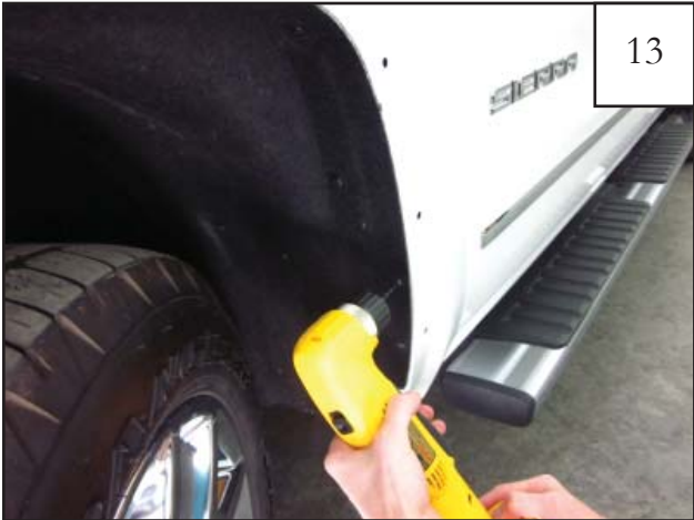
Remove the flare. Using a 3/32" drill bit, drill a pilot hole through the factory wheel well liner and sheet metal at location marked in previous step.
