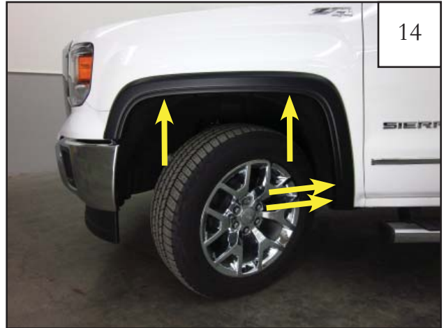
While holding Flare on vehicle, install supplied screws (SW1-0056) into the two upper and lower factory holes locations. Do not fully tighten at this time.
