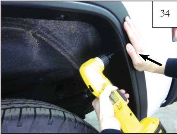
Install self-tapping screws (SW1-0066) into pilot holes drilled in step 31 (3 places). Press flare firmly towards the vehicle while fully tightening.
